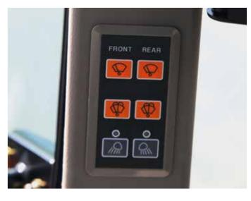
The control panel for lights and wiper is located on the right column so that all buttons are within easy reach of the driver.
