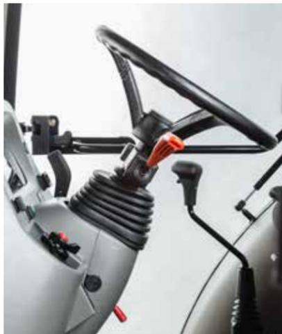
The HORTUS HS is equipped with a hydraulic reverser (PowerShuttle), which allows to conveniently change the driving direction without using the clutch pedal.
