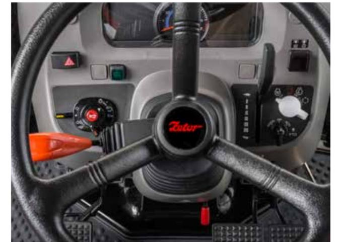
The easy-to-read LED dashboard displays operating data, such as engine speed, temperature, fuel level, time, PTO, etc.
