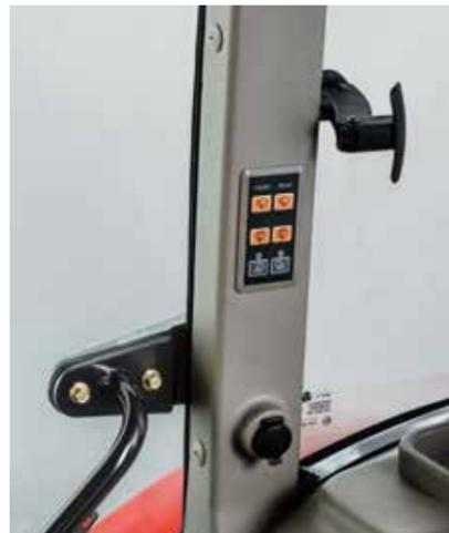
The control panel for lights and wiper is located on the right column so that all buttons are within easy reach of the driver.
