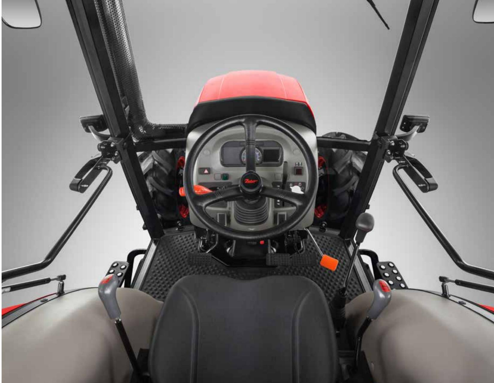
Wide doors allow the comfortable entry into the cab. The suspended seat, adjustable steering wheel and other ergonomic features ensure comfortable work.
