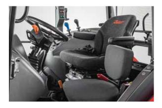
The Zetor seat provides ergonomical and comfortable sitting. Two seat options are available - seat with mechanical suspension or seat with pneumatic suspension. Each Proxima tractor is equiped with easily foldable and comfortable passenger seat with automatic safety belt.
