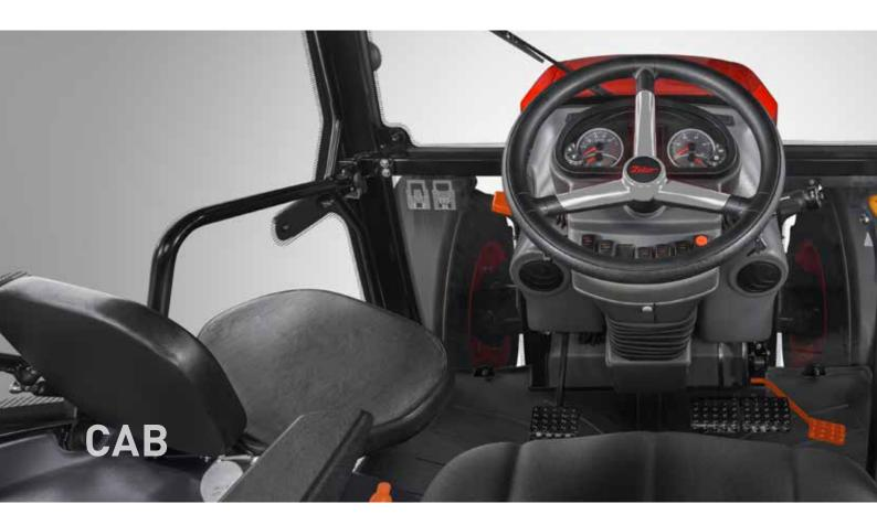
The cab is designed with regard to practical use. Plenty of space and ergonomically designed controls facilitate the work of the tractor operator. Optional equipment includes air-conditioning and radio. The opening roof hatch facilitates good cab ventilation and a good view. For work with the front loader, the cab can be equipped with a FOPS safety roof. As standard, the driver's and the passenger seats are fitted with safety belts.
